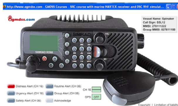
Rys. 3. Widok ogólny symulatora VHF DSC Fig. 3. General view of the VHF DSC simulator
